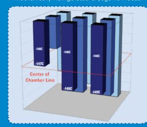
Comparison of temperature distribution in a liquid nitrogen freezer (vapor phase) and SANYO's MDF-C2156VANC mechanically refrigerated cryogenic freezer. Graph shows temperatures at different locations within the chamber. This data demonstrates that 100% of the MDF-C2156VANC storage space maintains uniform storage temperatures safely below -130°C, while temperature in LN<sub>2</sub> vapor system is dependent on storage location.
